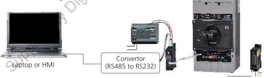
Most advanced release of MTX series, MTX3.0 is communication capable on MODBUS RTU network. Using MODBUS commodule the MCCB release can be connected to a Personal Computer. The metering values can be read remotely. The settings configuration on the other hand can both be read and changed remotely. These releases are also made compatible with HMI (Human Machine Interface) & DCS (Data Control Systems)
