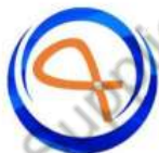
Min Bending Radius 5 ~ 6 Cable Diameter
