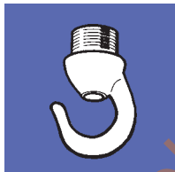
Hook, Male No. M502 Material: Malleable Iron Finishes: Black Enamel, Galvanised Size 20mm 25mm Standard Pack Qty 50 50
